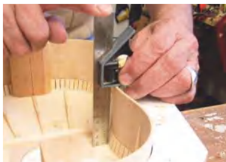
STEP 31. Ensuring opposite sides are equal height
